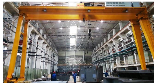
Double girder Gantry crane Max.200t
